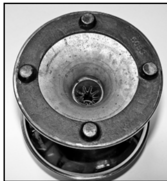
The P & A Sewing Lamp is center-draft with large wick tube. See metal heat exchange baffle in tube.
