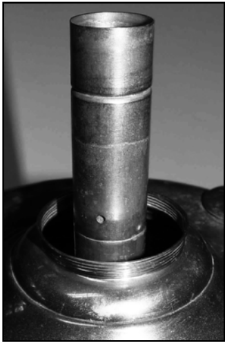
Model 6 wick tube showing one of three holes for drainage.
