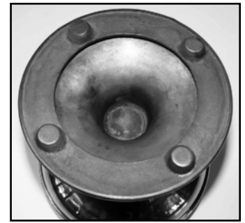
Plug in bottom of P & A Parlor Lamp to use for side-draft burners.
