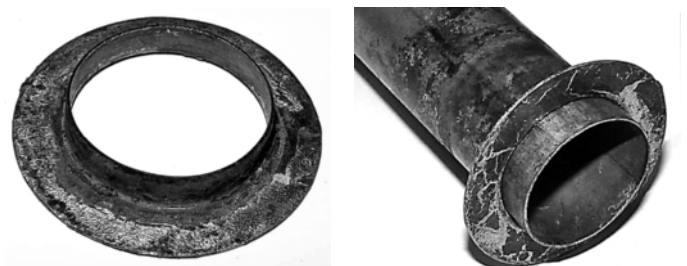
Collar fitting that is soldered into place to support the wick tube in the base of the fount. The tube usually extends below the collar.
